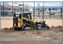
A skid steer with laser grader puts the finishing touches on the groundwork that will lie beneath the sod on the Little League Field at the new Dudley Key
